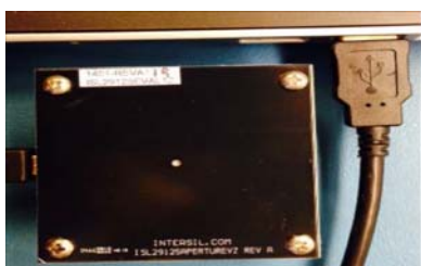
FIGURE 43. PC TO EVALUATION BOARD CONNECTION
