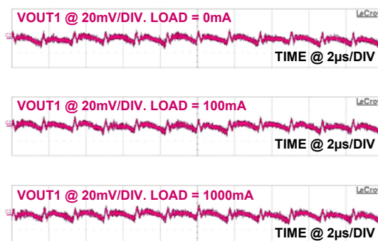
FIGURE 23. PWM1 OUTPUT RIPPLE, MODE = 5V (CCM)
