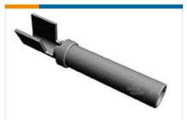
TE Part #776491-2 SOC, SF, SIZE 16, 14-18 AWG,NO INS, NI/SN
