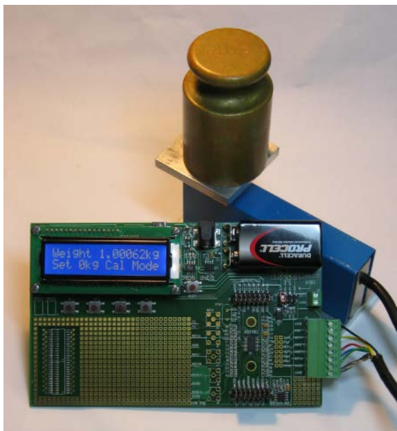
Figure 2. Weigh Scale System Using the AD7192
