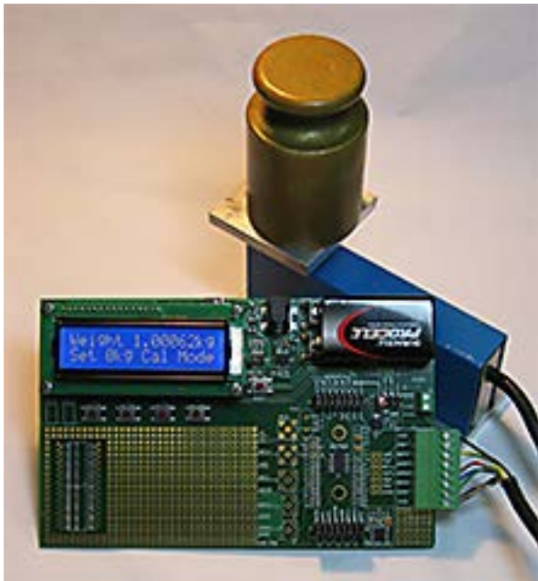
Figure 2. Weigh Scale System Setup Using the AD7190
