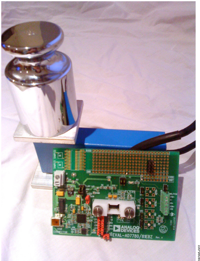
Figure 2. Weigh Scale System Using AD7781
