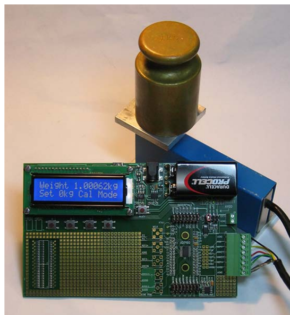
Figure 2. Weigh Scale System Setup Using the AD7195
