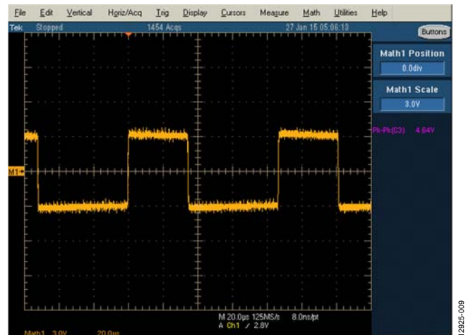
Figure 9. Math Y – Z Waveform for the RS-485 Port on the EVAL-CN0373-EB1Z Board
