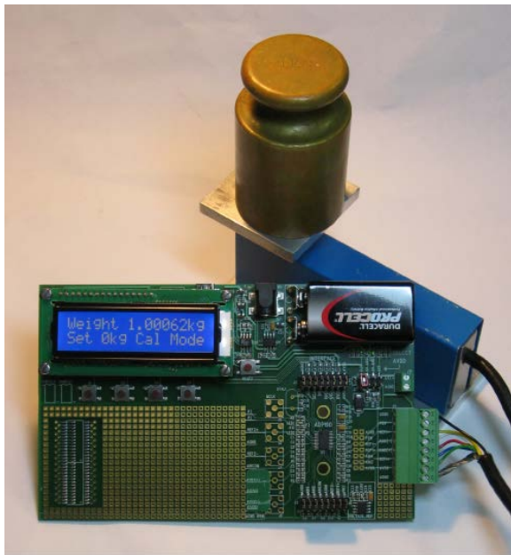
Figure 2. Weigh Scale System Using the AD7191
