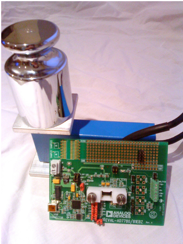
Figure 2. Weigh Scale System Setup Using the AD7780
