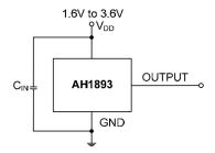
Note: 4. C<sub>IN</sub> is for power stabilization and to strengthen the noise immunity, the recommended capacitance is 100nF typical.
