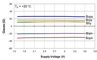
Switch Points vs Supply Voltage
