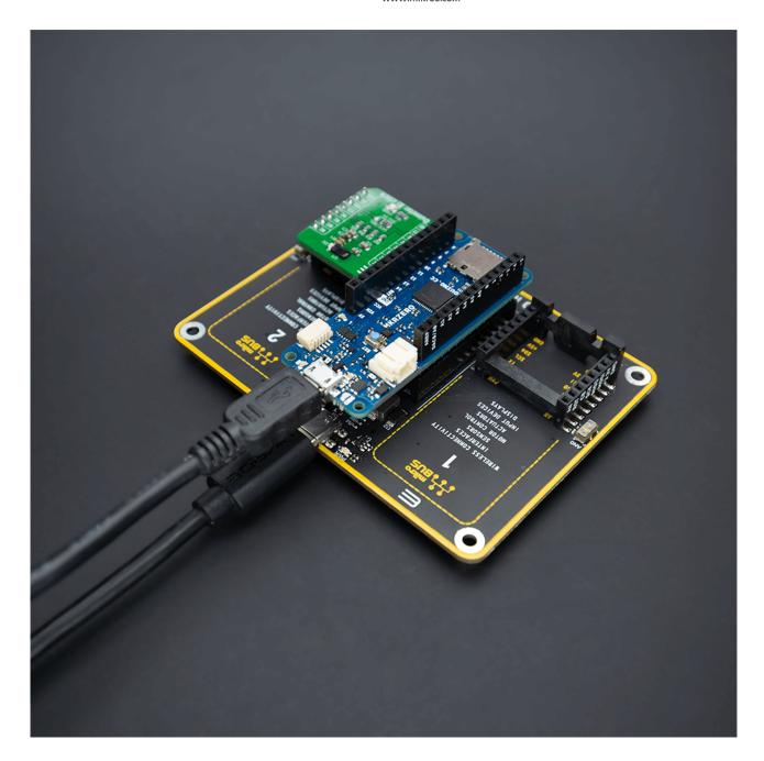
When the USB type C connector is connected to the Shield, and the other USB is connected to the Arduino MKR board, the PWR diode will glow Cyan, and at this setup, the mikroBUS™ sockets are powered from the Type C connector. The Arduino MKR board is unloaded from delivering power to them and is powered from its source (USB mini), over which you can also upload the program to your board.
