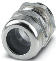
Cable gland, material for screw connection: Brass, nickel-plated, application: Standard, external cable diameter 18 mm ... 25 mm, shielding: no, connecting thread: Pg29, color: silver, with O-ring
