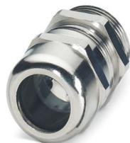
Cable gland, material for screw connection: Brass, nickel-plated, application: EMC, external cable diameter 18 mm ... 25 mm, shielding: yes, connecting thread: Pg29, color: silver, with O-ring
