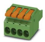
Plug component, nominal current: 41 A, rated voltage (III/2): 1000 V, number of positions: 4, pitch: 7.62 mm, connection method: Push-in spring connection, color: green, contact surface: Tin
