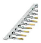
Crimp contact, Pin, rolled, Taped product, number of pieces per reel: 500, contact diameter: 1 mm, crimp range:  $0.22~\text{mm}^2$  ...  $0.56~\text{mm}^2$ , Item is lead-free in accordance with RoHS II without Exemption 6c (Pb < 0.1 %)
