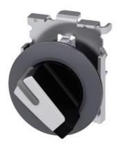
Selector switch, illuminable, 30 mm, round, Metal, matte, white, selector switch, short, front ring for flush installation, 2 switch positions O<I, momentary contact type, Actuating angle 45°, 10:30h/12h, with laser labeling, upper case and lower case, always upper case at beginning of line
