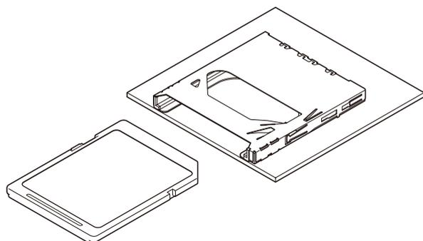
**This connector is designed for SD Card & MMC (Multi media card), complying with the SD Card Association standard, and is with the switch for Write-protection & Card-detection. And due to Push-push mechanism design, its card can be easily ejected by push-push operation.**
