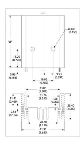
X Dim: 15.88 (0.625) | Y Dim: 2.64 (0.104) | Z Dim: 2.67 (0.105)
