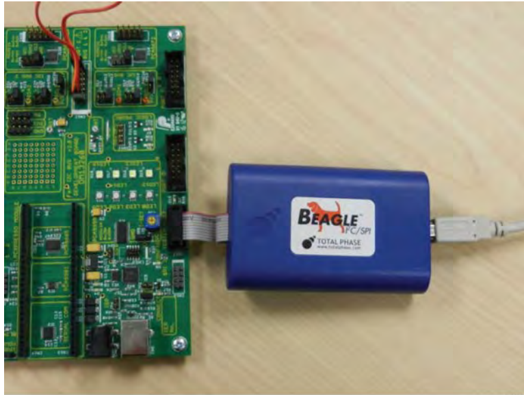
Fig 82. Beagle Bus Logger connected to the Fm+ development board (OM13260)
