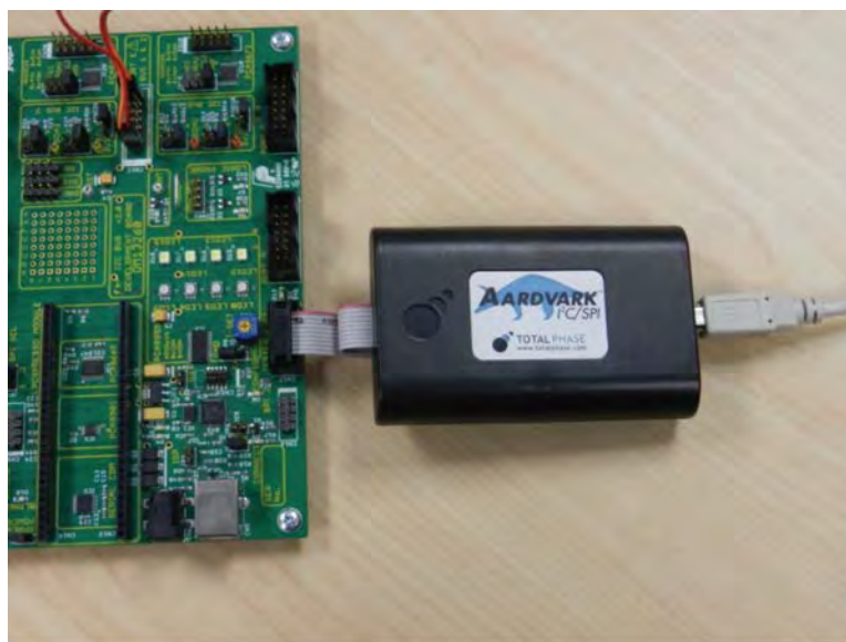
Fig 81. Aardvark Host Adapter connected to the Fm+ development board (OM13260)
