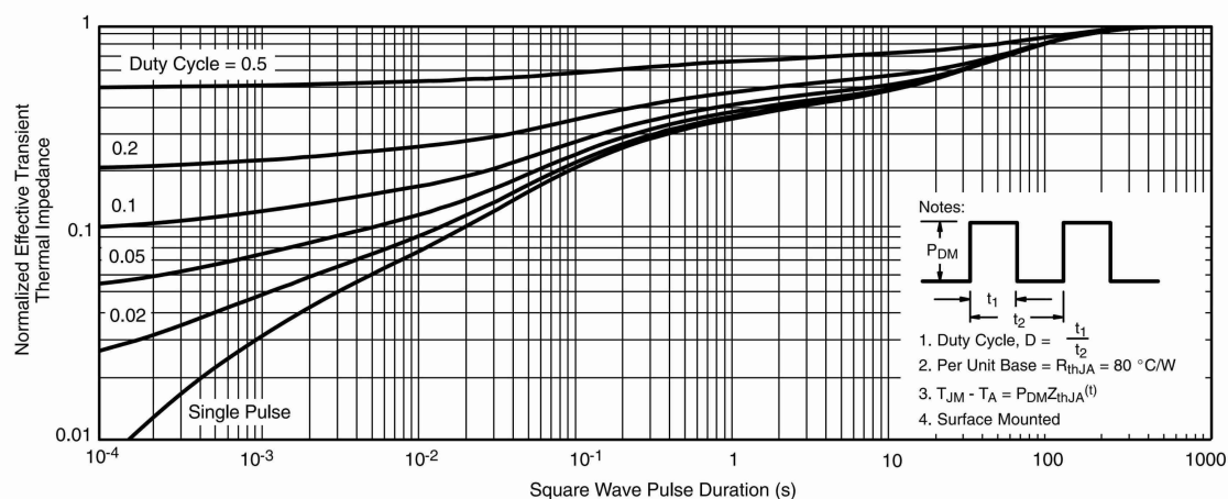
Normalized Thermal Transient Impedance, Junction-to-Ambient
