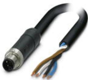
Power cable, 4-position, PVC, black-gray RAL 7021, Plug straight M12, L-coded, on free cable end, cable length: 10 m, for direct current up to 16 A/63 V
