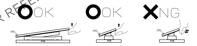
(3) IF THE FPC IS NOT RIGID, THE CONNECTOR CAN BE BROKEN. PLEASE CHECK THE ACTION OF THE FPC TO BE USED REPEATEDLY AT THE TIME OF TRIAL PRODUCTION. BE CAREFUL TO UN-MATE THEM FROM THE PITCH DIRECTION. PULLING IT FROM THE CORNER CAN ALSO RISK TO PUTTING STRESS ON CONTACTS.
