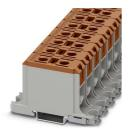
High-current terminal block, nom. voltage: 1000 V, nominal current: 145 A, number of connections: 2, number of positions: 1, connection method: Screw connection, Rated cross section: 50 mm<sup>2</sup>, cross section: 6 mm<sup>2</sup> - 50 mm<sup>2</sup>, Rated cross section: 50 mm<sup>2</sup>, cross section: 4 mm<sup>2</sup> - 50 mm<sup>2</sup>, mounting type: NS 35/15, NS 35/7,5, color: brown
