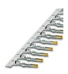
Crimp contact, Socket, rolled, Taped product, number of pieces per reel: 500, contact diameter: 1 mm, crimp range:  $0.22~\text{mm}^2$  ...  $0.56~\text{mm}^2$ , Item is lead-free in accordance with RoHS II without Exemption 6c (Pb < 0.1~%)
