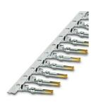
Crimp contact, Socket, rolled, Taped product, number of pieces per reel: 10000, contact diameter: 1 mm, crimp range:  $0.22~\text{mm}^2$  ...  $0.56~\text{mm}^2$ , Item is lead-free in accordance with RoHS II without Exemption 6c (Pb < 0.1~%)
