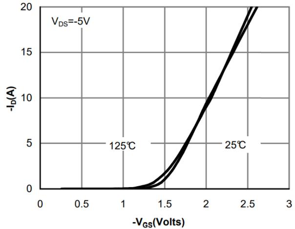
**Figure 2: Transfer Characteristics**
