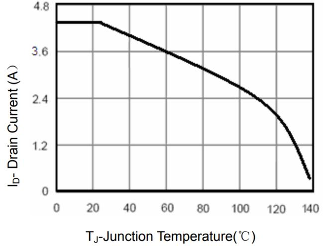
Figure 10: Drain Current
