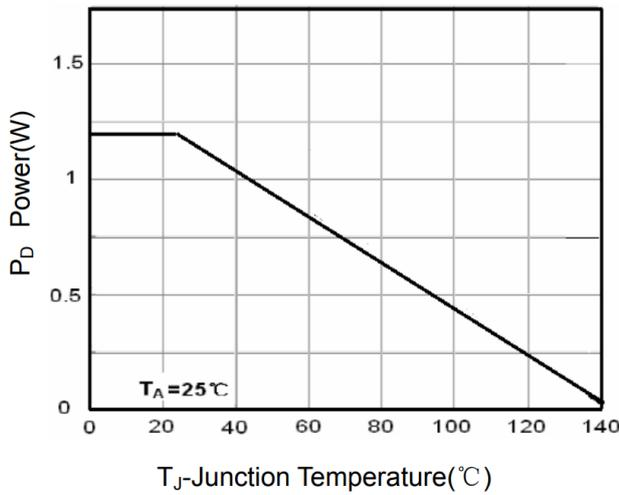
Figure 9: Power Dissipation
