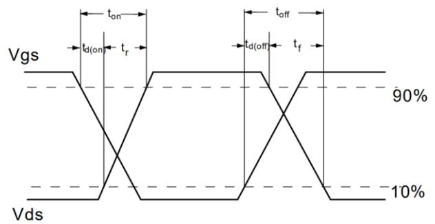
Figure 12: Switching Waveform
