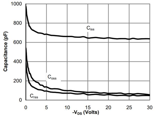
Figure 8: Capacitance Characteristics
