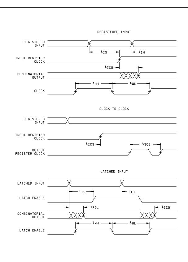
FIGURE 4. Switching waveforms - Continued.
