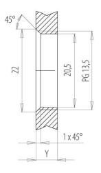
Installation direction: o-ring sits on chamfer.
