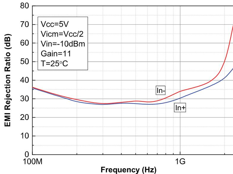
EMIRR performances might be improved by adding small capacitances (in the pF range) on the inputs, power supply and output pins. These capacitances help minimize the impedance of these nodes at high frequencies.
