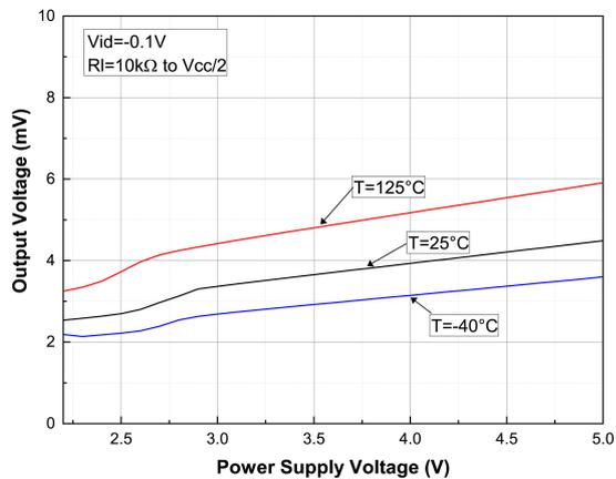
Figure 18. Output saturation voltage ( $V_{OH}$ ) vs. supply voltage
