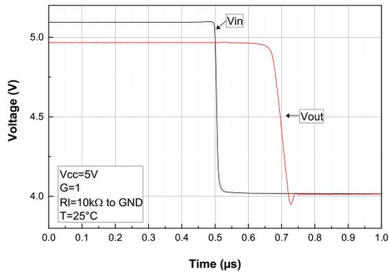
Figure 32. Small step overshoot vs. load capacitance
