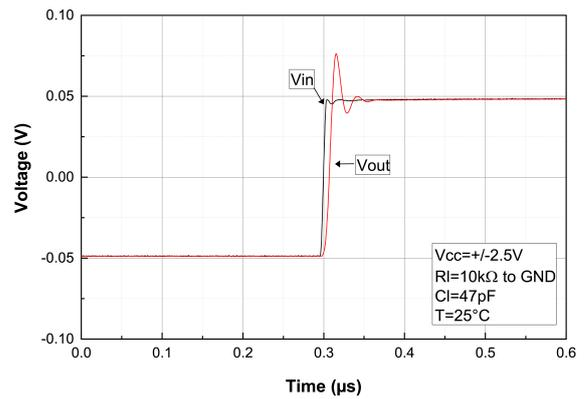
Figure 29. Small step response at  $V_{CC} = 2\text{ V}$
