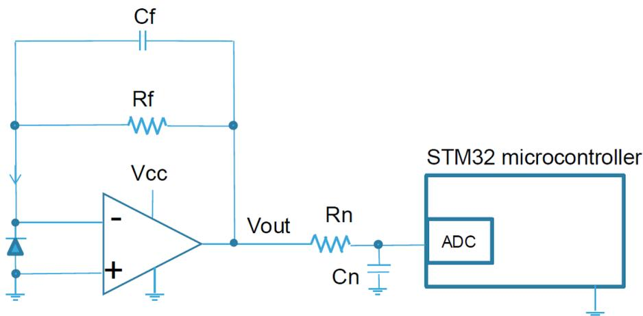
The transimpedance amplifier circuit converts the small photodiode output current in the nA range, into a voltage signal readable by an ADC following Eq. (13):
