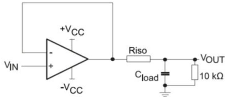
Please note that  $R_{ISO} = 22 \Omega$  is sufficient to make the TSV78x stable whatever the capacitive load.
