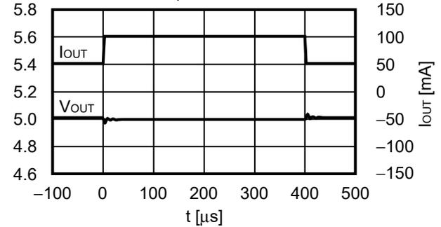
3. Load dump characteristics ( $T_a = +25^\circ\text{C}$ )
