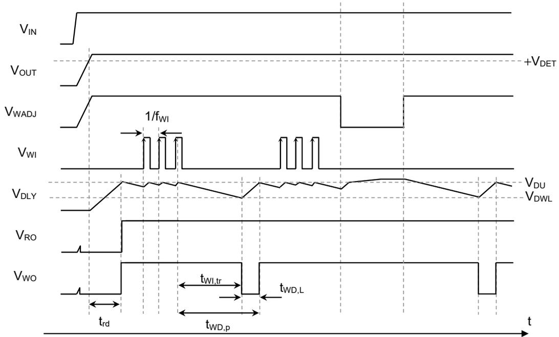
**Figure 42 Example of Watchdog Timer Monitoring Operation**
