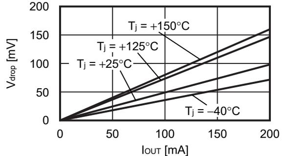
**1.4 Dropout voltage vs. Junction temperature**
