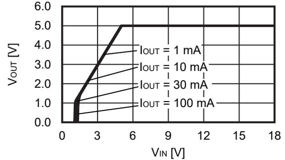
**1.3 Dropout voltage vs. Output current**
