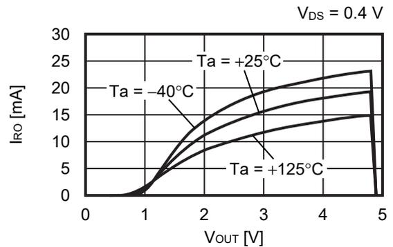
**2.5 RO pin voltage vs. Output voltage**
