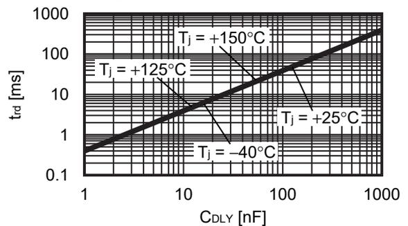
**2.8 Reset reaction time vs. Junction temperature**
