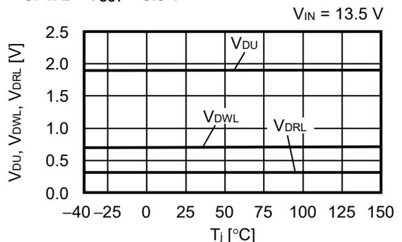
**3. 5 Watchdog activation threshold current, watchdog deactivation threshold current vs. Junction temperature**
