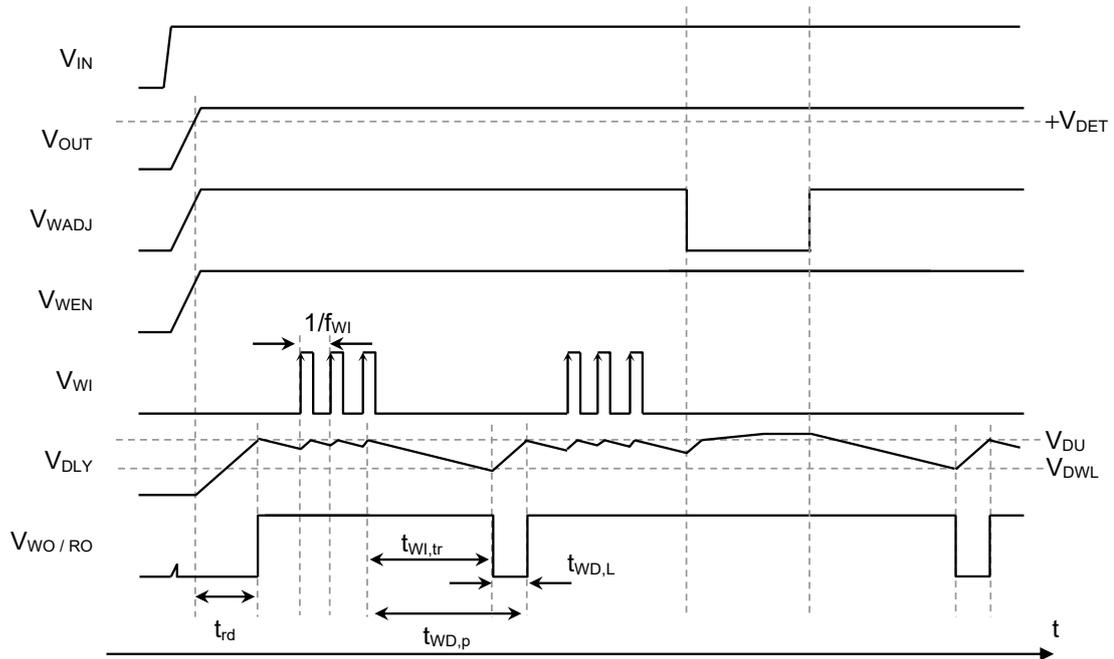
**Figure 39 Example of Watchdog Timer Monitoring Operation 1**
