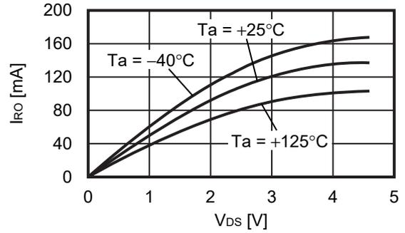
**2.4 Reset output current vs. Output voltage**
