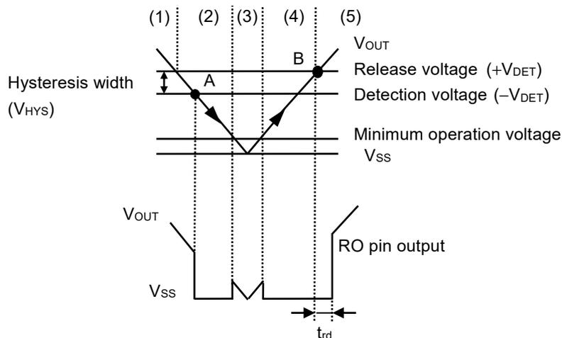
**Figure 34 Timing Chart of Detector Block**
