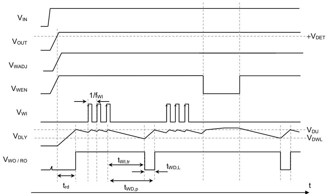
**Figure 40 Example of Watchdog Timer Monitoring Operation 2**
