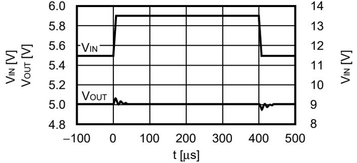
2. Characteristics of load transient response ( $T_a = +25^\circ\text{C}$ )
