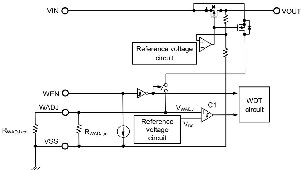
**Figure 37 Operation of Output Current Detection Circuit**
