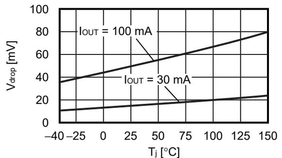
**1.5 Output voltage vs. Junction temperature**
