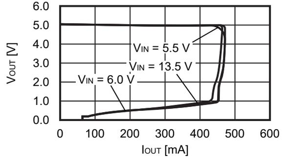
**1.2 Output voltage vs. Input voltage (Ta = +25°C)**
