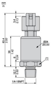
(1) SW24, tightening torque  $\leqslant$  24 N-m / 212 lb-in
