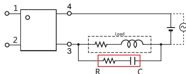
When adding diodes, buffer circuits (C-R), and other protections, they need to be installed near the MOS RELAY to be effective.
