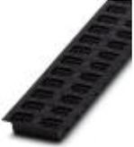
Header, Nominal current: 8 A, Rated voltage (III/2): 160 V, Number of positions: 9, Pitch: 3.5 mm, Color: black, Contact surface: Tin, Mounting: THR soldering, User information and design recommendations for through hole reflow technology can be found under "Downloads"
