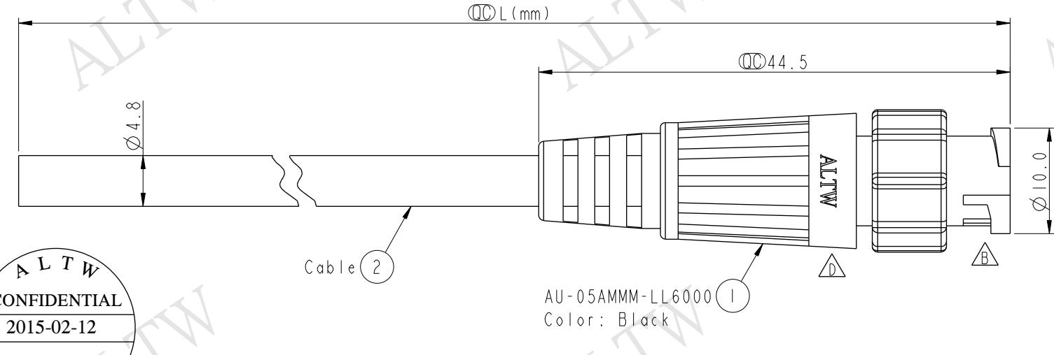
Front View Drawing showing dimensions: ØD L (mm), ØD 44.5, Ø 4.8, Ø 10.0. Part number AU-05AMMM-LL6AXX. Color: Black. Pin assignments: 1 (Green), 2 (Brown), 3 (Red), 4 (White), 5 (Yellow). Cable length tolerance: 01~99Meters. Connector type: AU-05AMMM-LL6000 Conn.
