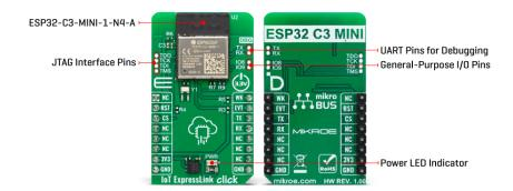
The IoT ExpressLink Click interfaces with a host MCU through UART communication, which involves sending AT commands using RX and TX pins operating at a rate of 115200bps. Besides the UART pins, this Click board™ also employs other pins of the mikroBUS™ socket to enhance its functionality. For example, the WK pin is utilized as a module wake-up pin, the EVT pin detects significant events during operation, and the device enable pin RST offers a switch operation to turn ON/OFF the module.
