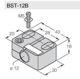
Mounting clamp for threaded barrel sensors, with dead-stop; material: PA6
