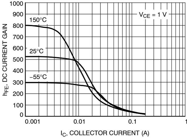
Figure 1. DC Current Gain vs. Collector Current
