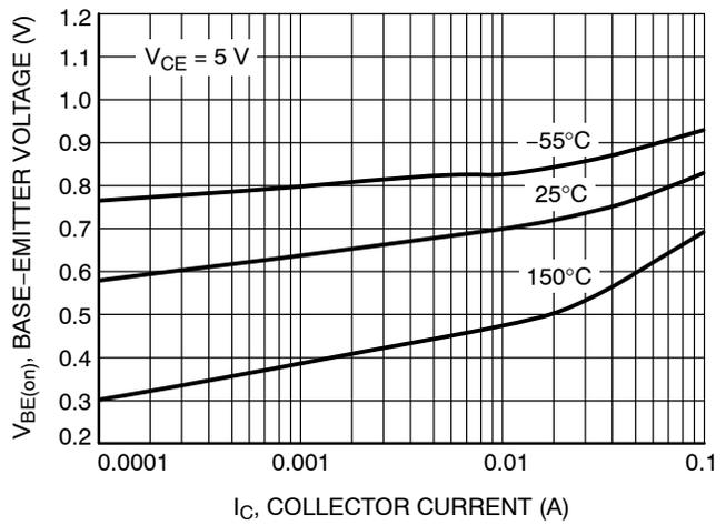
Figure 4. Base Emitter Voltage vs. Collector Current
