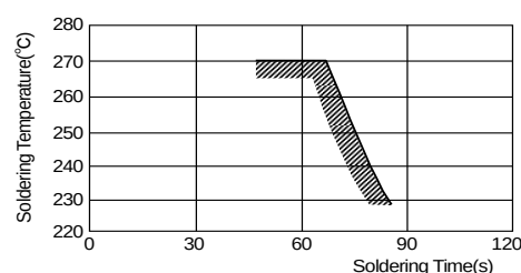
[Allowable Reflow Soldering Temperature and Time]
