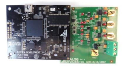
The AD5453 is a CMOS 14-bit current output digital-to-analog converters, respectively. These devices operate from a 2.5 V to 5.5 V power supply, making them suited to several applications, including
