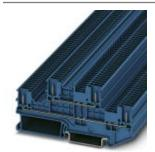
Double-level terminal block, Cross section: 0.14 mm² - 1.5 mm², AWG: 26 - 14, Connection type: Plug-in connection, Width: 3.5 mm, Color: blue, Mounting type: NS 35/7,5, NS 35/15
