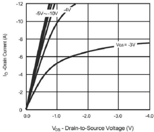
Figure 1. Output Characteristics
