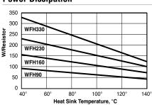
This graph shows the maximum wattage rating for each possible resistor of standard size corresponding to the heat sink temperature. It is assumed that all resistors are equally loaded.
