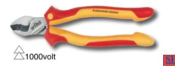
328 Serrated Edge Cable Cutters. Insulation According to VDE 0682/part 201, EN/IEC 60900, ASTM F-1505-01, NFPA70E and CSA, A up to 1000 Volt. Individually Tested. Light, clean cutting ground precision cutting edges. Durable cutting is achieved through additional inductive hardening to approx. 64HRC. Special tool steel, hardened & tempered. For cutting of copper & aluminum cables without crushing.
