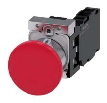
Mushroom pushbutton, 22 mm, round, metal, shiny, red, 40mm, latching, pull-to-unlatch mechanism, with holder, 1 NO+1 NC, screw terminal, with laser labeling, inscription or symbol Customer-specific selection with SIRIUS ACT configurator (CIN)
