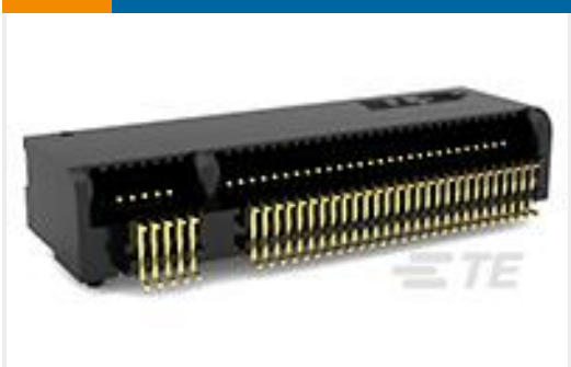
TE Part #2199230-8 M.2 0.5PITCH 4.2H KEY A 15U" AU
