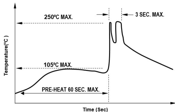
**NOTE:** Figure 9 refers to measurements with thermocouple mounted at the bottom of the PCB.
