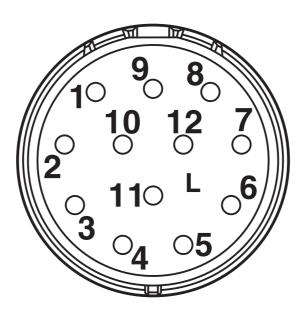
Contact chamber numbering (view of plug-in side), standard socket
