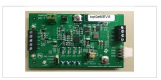
2 Series, 3 Series, and 4 Series Li-Ion Battery Pack Manager Evaluation Module
