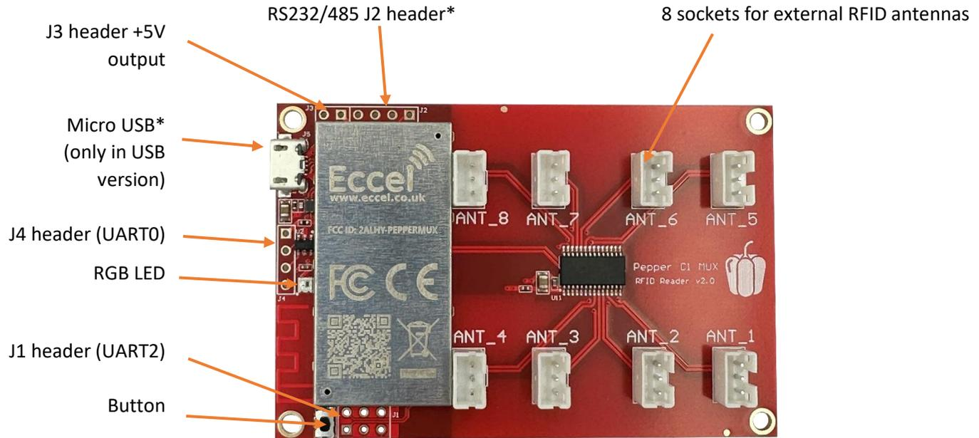
\*Micro USB – only in USB version. Connected internally to the built in USB to TTL converter. This converter is routed to the UART0 header.
