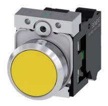
Pushbutton, 22 mm, round, metal, shiny, yellow, pushbutton, flat, momentary contact type, with holder, 1 NO, screw terminal, with laser labeling, upper case and lower case, always upper case at the beginning of the word
