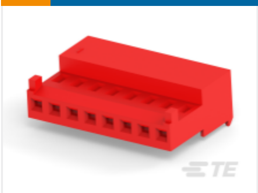
TE Part #3-644042-3 Nylon Gold Plated Receptacle: 2.54 mm, with Mating Alignment, MTA 100
