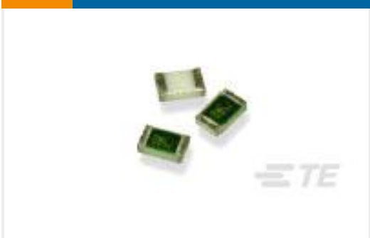
TE Part #8-1614884-4 CPF 0805 10K 0.1% 25PPM 1K RL
