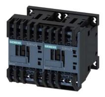
Reversing contactor assembly AC-3, 3 kW/400 V 110 V AC 50 Hz/120 V 60 Hz, 3-pole Size S00, Spring-type terminal electrical and mechanical interlock
