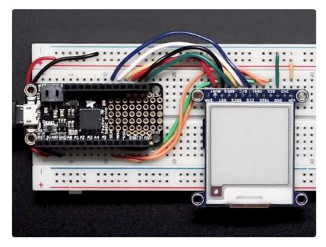
One thing to remember with these small e-lnk screens is that its very slow compared to OLEDs, TFTs, or even 'memory displays'. It will take may seconds to fully erase and replace an image
