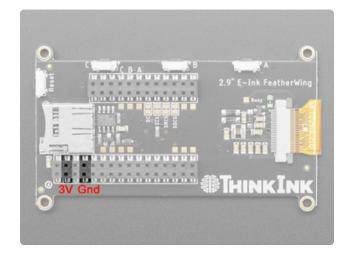
3V - this is the power pin, and connects to the Feather 3V power supply outputGND - this is the power and signal ground pin
