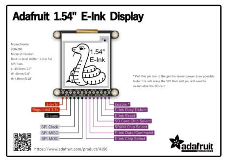
The pin outs are identical for the 1.54", 2.13" and 2.7" E-lnk display!
