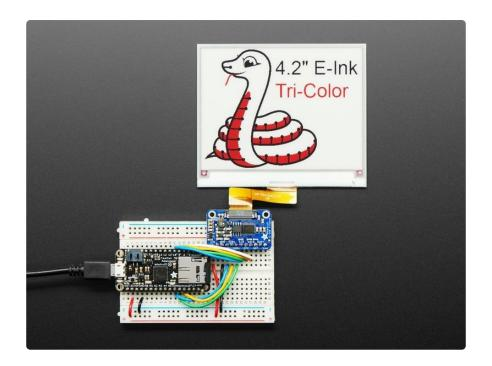
On the Elnk Friends and Breakouts, for ultra-low power usages, the onboard 3.3V regulator has the Enable pin brought out so you can shut down the power to the SRAM, MicroSD and display.
