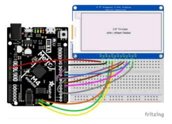
Vin connects to the microcontroller board's 5V or 3.3V power supply pin GND connects to ground CLK connects to SPI clock. It's easiest to connect it to pin 3 of the ICSP header. MOSI connects to SPI MOSI. It's easiest to connect it to pin 4 of the ICSP header.
