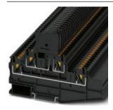
Fuse modular terminal block, Connection method: Push-in connection, Cross section:  $0.2 \text{ mm}^2$ -  $6 \text{ mm}^2$ , AWG: 24 - 10, Nominal current: 28 A, Nominal voltage: 500 V, Width: 6.2 mm, Fuse type: G /  $5 \times 20$ , Fuse type: Glass / ceramics / ..., Mounting type: NS 35/7.5, NS 35/15, Color: black
