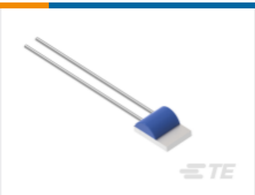
TE Part #NB-PTCO-046 Pt1000, 2.0x2.3, Class C, PTFC102C1G0
