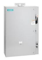
Pump control panel, Size 3, Three phase full voltage, Solid-state overload relay, OLR amp range 25-100A, 110-120/220-240VAC 60Hz coil, Standard type contactor, 200A fusible disconnect, 200A/250V fuse clip, HOA Sel Sw. & Start P.B., Enclosure NEMA type 3/3R, Weather proof outdoor use
